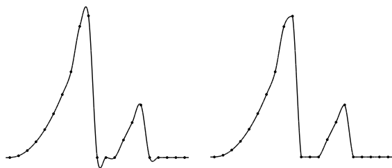
Figure 9: Standard cubic Hermite interpolation (left) produces overshoots while our modified interpolation scheme (right) guarantees that no overshoots occur.
