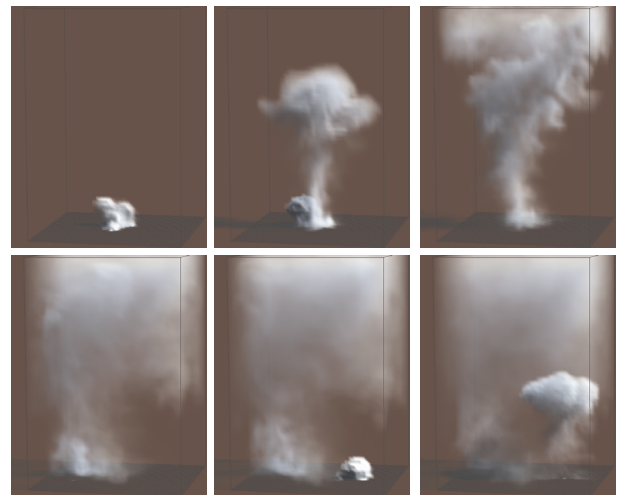
Figure 7: Six frames rendered using our interactive hardware renderer of the smoke. The simulation time for a 40x40x40 grid was roughly 1 second/frame.
